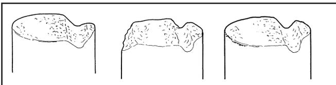
As the next illustration shows, fatigue failures take many forms, but they all exhibit similar features. Generally, the broken surface is brittle and has a "lip" like that in the bending failure, even though, in some cases, the lip has been broken.
