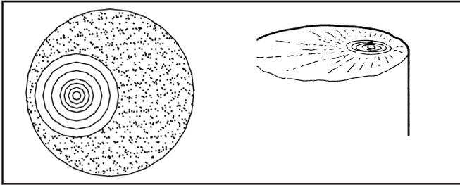
As a rule, working steel failures can be diagnosed by looking at the break itself, and at the place on the steel where the break occurred. Discoloration, like “rainbow” effects or blue bands, is the result of extreme heat.
