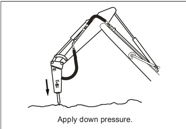
Apply down force to the boom/dipper until the rear of the backhoe is raised off the ground. Rear tires and stabilizers should be off the ground so the total rear weight of the backhoe is on the breaker tool. The breaker is more efficient when adequate down force is applied.
