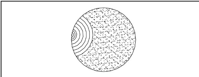
Similar failures can also occur when the steel is used with extreme down pressure, and the steel repeatedly slips off the work at an angle, or the material, itself moves from under the working steel.
