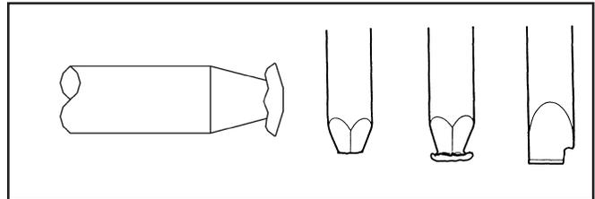
If the overheated steel is suddenly cooled by being dipped in standing water, for example, the metal will harden and become brittle. These are some examples of failure caused by temper changes occurring on the job.
