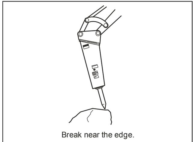
On flat material or rock, the breaker should be vertical or “curled” back slightly to direct the impact force downward and toward the backhoe. This directs the force back toward the edge of the work material. If the tool is positioned in the center of the work, or too far from the edge, the energy will be absorbed into the material without cracking it. Do not run the breaker longer than
