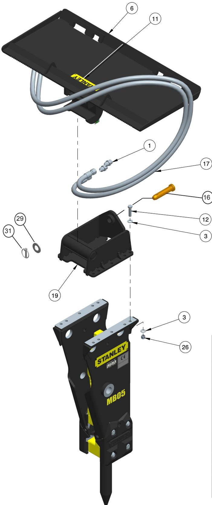
NOTE: The MB05S04 comes with 2 additional Adapters P/N-02773 not pictured. Also comes with a male coupler P/N-40092 and Female coupler P/N-65811 that are also not pictured. See parts list below.
