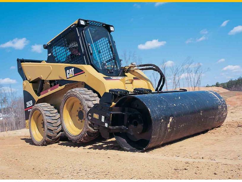
A hydraulically powered vibrating roller used to compact soil, stone and asphalt.
