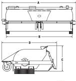
**BP15B and BP18B Pickup Brooms** Options: Bolt on cutting edge, polly/wire replacement bristles, machine mounted water tank, gutter brush. For building sites, general utility, parking lot.
