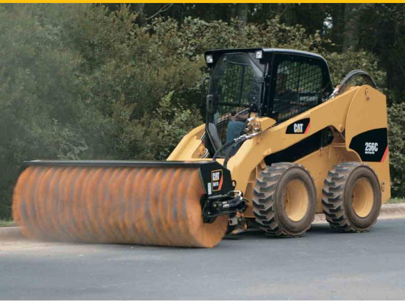
A range of angle and pickup brooms for use in construction, industrial and recycling applications.
